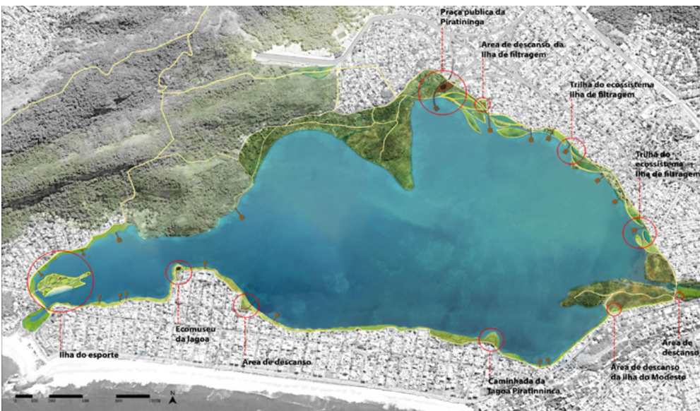
Figure 50. Plan of the parks with wetlands to filter run-off before it reaches the lagoon and location of various uses and equipment.
