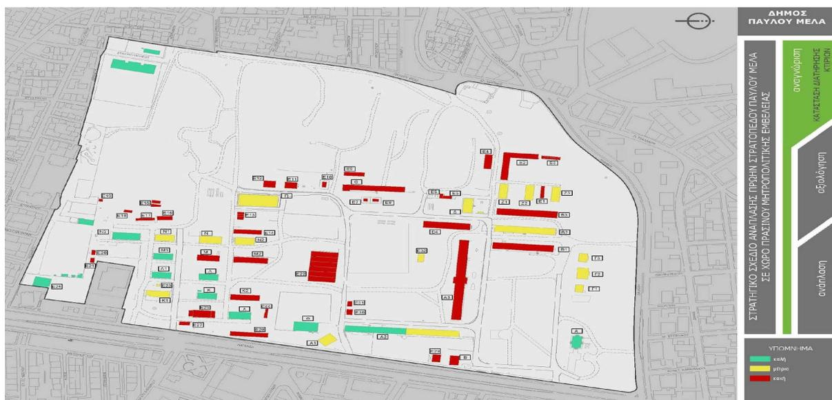
Figure 8: Building stock: 24.292 m<sup>2</sup> built surface. Green-16% (4.115 m<sup>2</sup>) in good condition, Yellow-26% (6.531 m<sup>2</sup>) in moderate condition and Red-58% (13.646 m<sup>2</sup>) in bad condition
